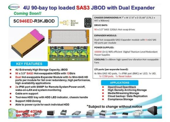
One very neat feature of the JBOD is it has 2 x Hot S wappable expander modules with 4 x Mini-SAS HD ports per module to give you fail over redundancy and high application performance. Also includes 2 x IPMI ports for remote system management.
