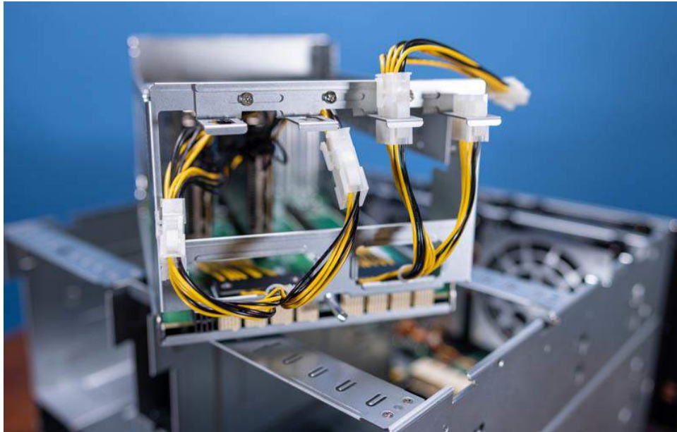
AIC JBOX J5010 02 Two Xilinx U55 Based FPGAs Installed With Consumer GPU Connector
