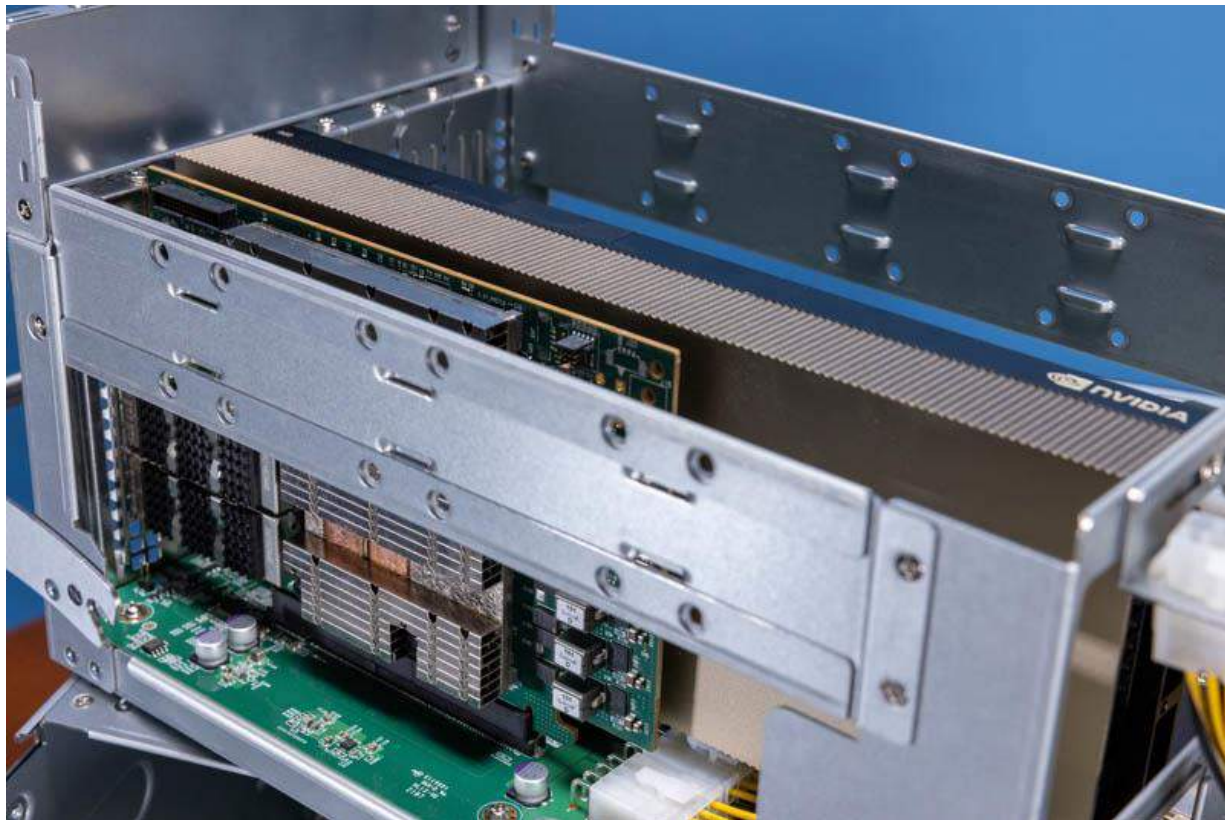
AIC JBOX J5010 02 NVIDIA BlueField 2 And A40 Installed 2
