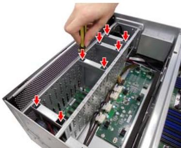
7. Lift up the HDD cage from the chassis
