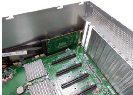
2. Screw the GPU bracket to the GPU card and connect the GPU PWR cable.
