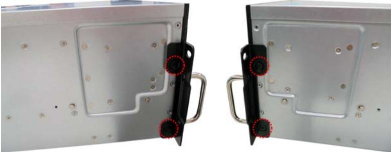
2. Press the latch key to draw out the inner rails from sliding rails.
