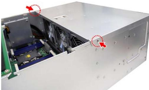
4. Release the latch to lift up the front top cover from the chassis.
