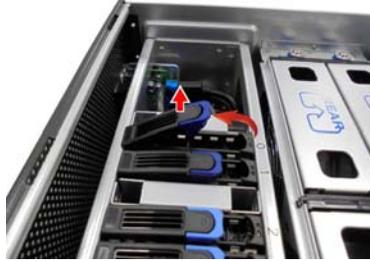
2. Remove 4 screws to detach the HDD tray bracket.
