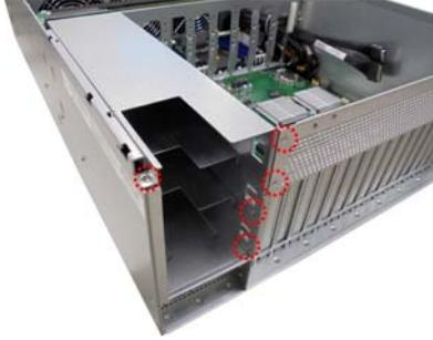
2. Unscrew the power supply cage.
