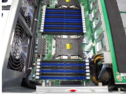
3. Refer to Section 3.9 Replacing the Riser Card and 3.10 Replacing the Power Backplane Board to remove the Power Supply Cage and the PBP Tray.
