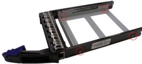
3. Place a HDD/SSD into the drive tray. Use four screws to secure the HDD/SSD.
