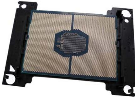
2. Carefully flip the heatsink. Then install the carrier assembly on the bottom of the heatsink and make sure the gold arrow is located in the correct direction.
