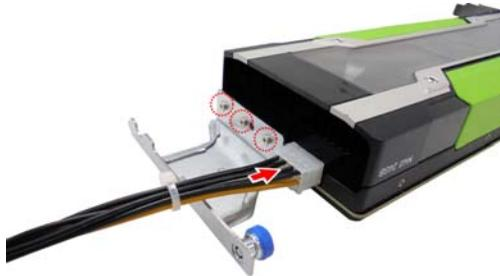
3. Insert the GPU card into the PCIE Gen. 3 slot and screw the GPU card to the chassis. Connect the GPU PWR cable to the Power Distribution Board.
