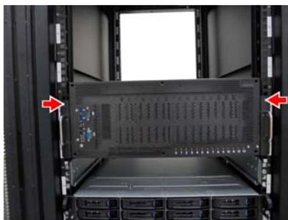
4. Press the latch keys on both sides simultaneously to pull the system out.
