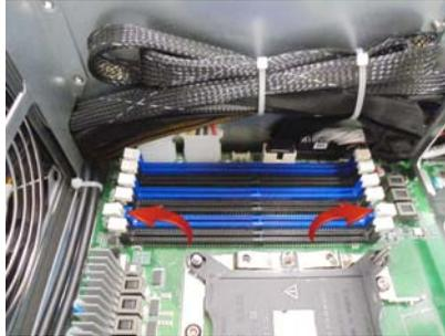
2. Align the memory module with the slot. When inserted properly, the memory slot locking levers lock automatically onto the indentations at the ends of the module.
