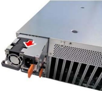
3. Replace a new single power and reinsert it into the power cage following the above steps in reverse.
