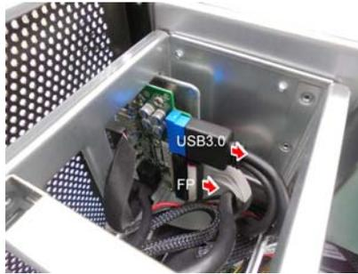
2. Unscrew to remove the front panel board module.
