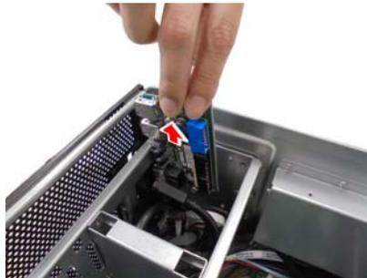
3. Loosen three screws to take out the front panel board. Remove the ID Button cap, LED sponge and LED Lens to reinstall in the new Front Panel Board.
