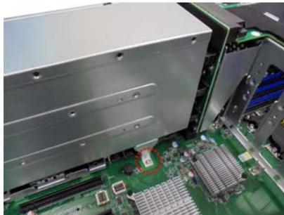
3. Lift up the power supply cage.
