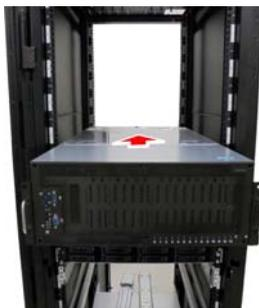
3. Screw the mounting ears of chassis to the rack.
