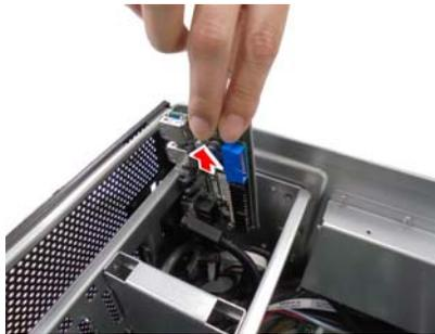
4. Unscrew the Front COM and VGA Ports.
