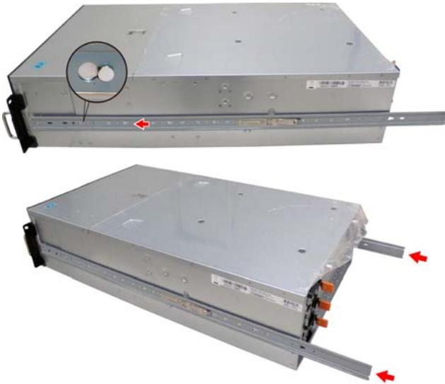
4. Secure the screws to both sides of the chassis.
