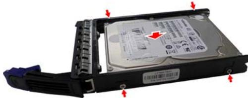
4. Reinsert the HDD tray into the HDD cage.
