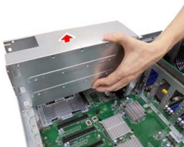
4. Loosen the screws to lift up the bracket.
